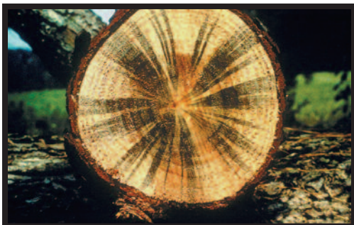
Blue stain fungus penetration in Southern Pine log cross-section
